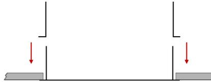
**STEP 3** - Block the frame on false ceiling with 2 L brackets, then connect the lamp to line 220Vac and fix it to the frame using the screws supplied.
