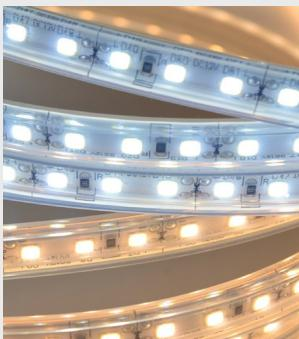
HS9 is a flexible LED strip, very thin and suitable for lighting application and luminous decoration.
