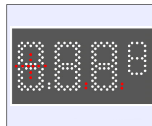
Additional LEDs and functions for + symbol or decimal points in a position other than the standard **
