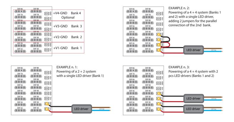
The two jumpers: positive (red wire) and negative (black wire) are used to connect 2 banks in parallel to the same LED driver.
